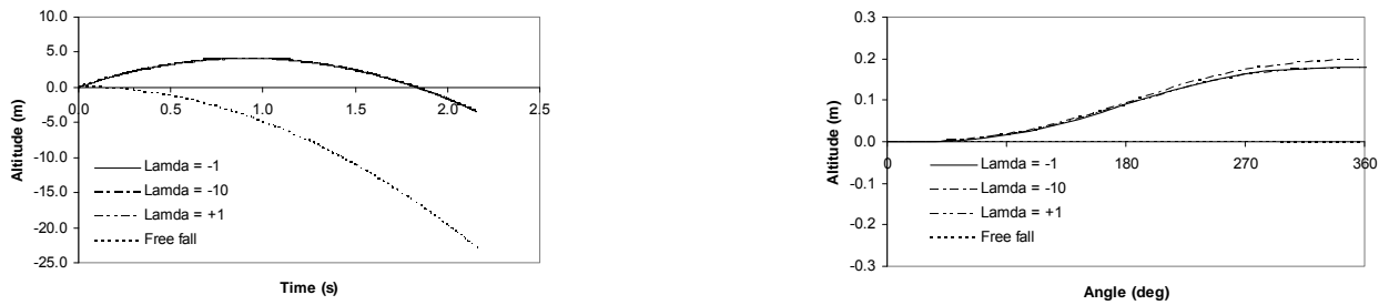
Figure 4: Vertical displacement z_M(t) versus time for the first four rounds of the rigid rods (left) and the first one (right)
